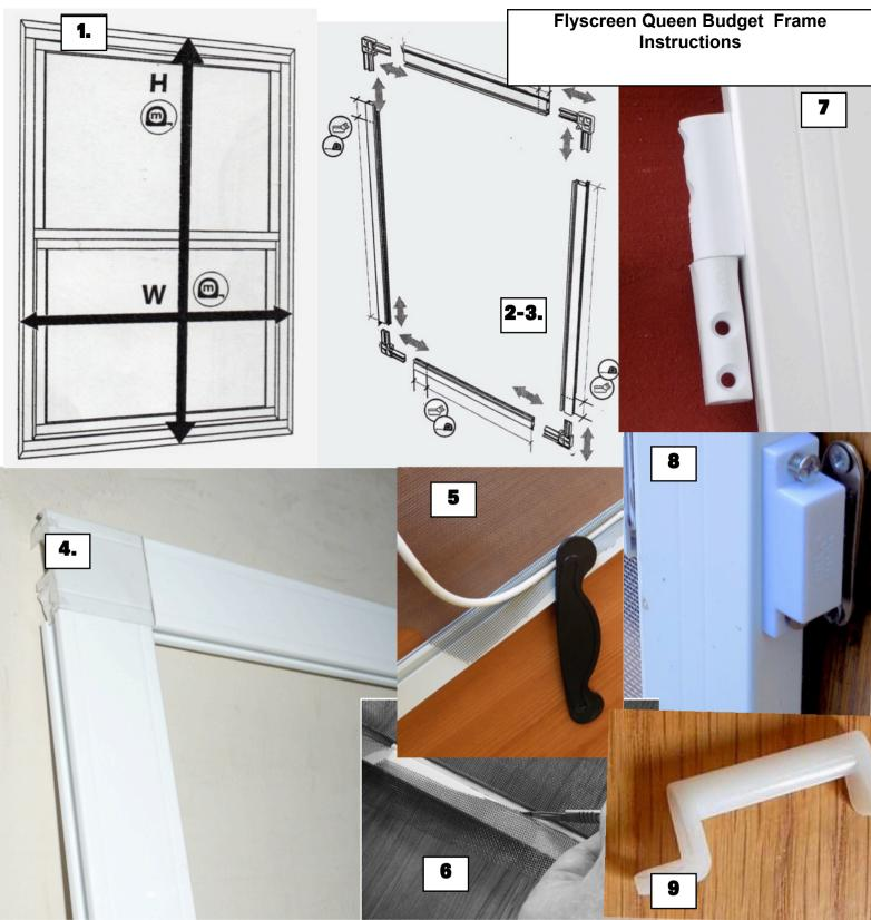
What you Get • Profiles x 4 • Rubber Spline • Grey Flyscreen Material • Corners x 4 • Handles x 1 • Hinges x 2 + Screws You will Need • Drill • Large Rubber Mallet • Hacksaw/Mitre Box or Mitre Saw • Crosshead Screwdriver • Glue
