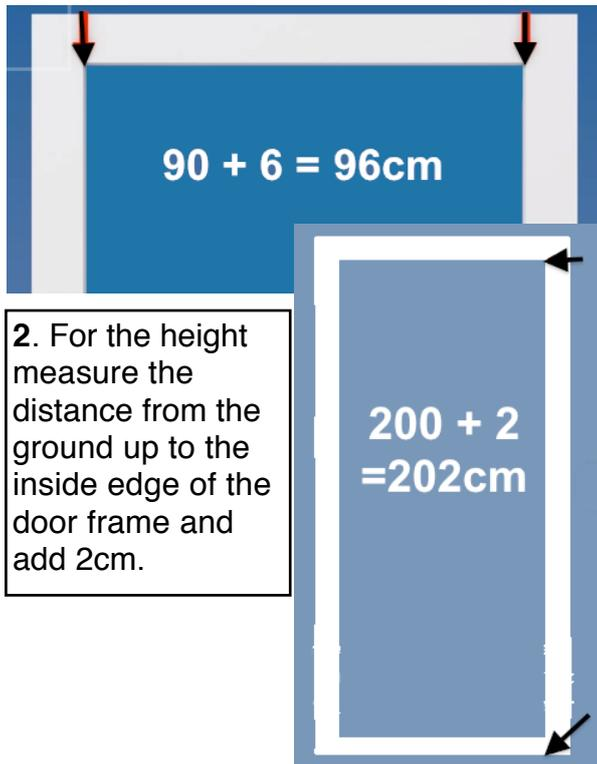
2. For the height measure the distance from the ground up to the inside edge of the door frame and add 2cm.
