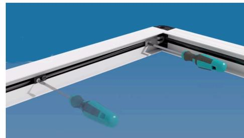
7. Once you have assembled the flyscreen frame you can now raise it into place. This is a two person job. Position and then screw into the frame work of your doorway with the four screws provided. Now attach the plastic covers over screw holes.
