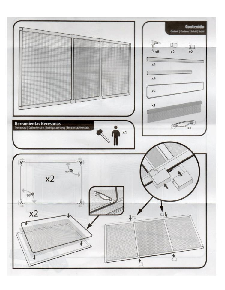
Sash Assembly Tips Make Sure the Frames are facing the right way with all the grooves on the same side. This also applies to the corners.
