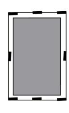
SECURE THE MATERIAL IN THE FRAME PIECES BY FOLDING THEM OVER- YOU CAN APPLY HAND PRESSURE BUT A MALLET IS EASIER AND QUICKER-
